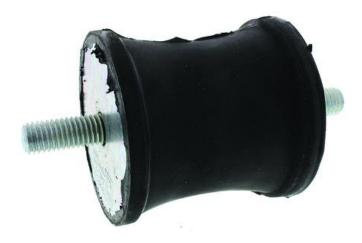
Their elasticity is much greater in all the directions parallel to the armatures than in the perpendicular direction. The rubber works based on compression or shear depending on the direction it is placed in at installation time. This direction is made according to the use and the objective.
