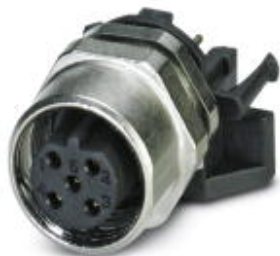
Sensor/actuator flush-type socket, 5-pos., M12 SPEEDCON, B-coded, rear/screw mounting with M12 thread, with polarity protection, with straight solder connection
