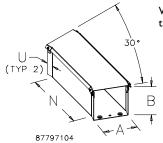
When a large radius is needed, use this sweep elbow.
