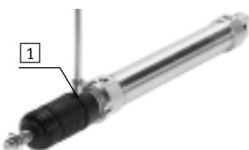
The bellows kit is a leak-free system. To prevent unwanted media from being drawn in, the supply and exhaust air of the kit must be ducted via a pressure compensation hole in the connection section [1].
