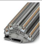
Double-level terminal block, Cross section: 0.14 mm² - 1.5 mm², AWG: 26 - 14, Connection type: Push-in connection, Width: 3.5 mm, Color: gray, Mounting type: NS 35/7,5, NS 35/15
