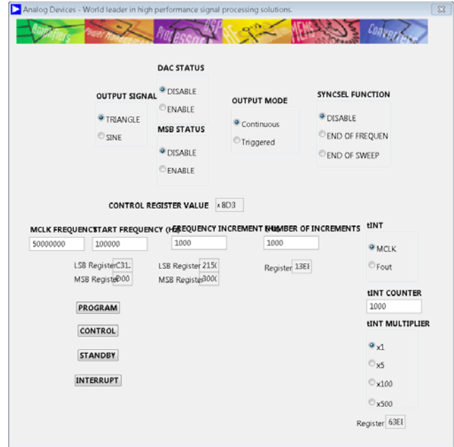
Figure 2. LabView GUI for AD5932
