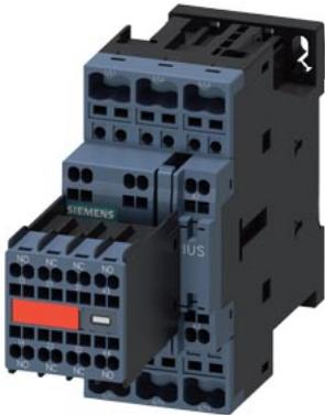
power contactor, AC-3e/AC-3, 9 A, 4 kW / 400 V, 3-pole, 230 V AC, 50/60 Hz, with plugged-in varistor, auxiliary contacts: 2 NO + 2 NC, spring-loaded terminal, size: S0, captive auxiliary switch
