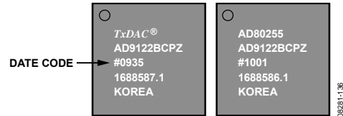
Figure 36. Revision 1 Silicon, AD9122BCPZ Marking
