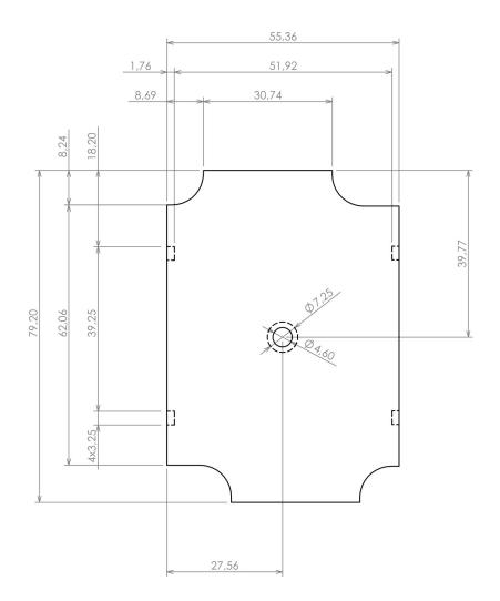
Dashed line shows outline of the mounting boss under PCB board Recommended mounting holes diameter ø4mm All dimensions are given within +/-0,5mm tolerance
