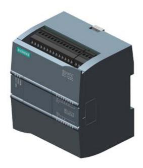
KOMPAKT CPU, DC/DC/RELAIS, ONBOARD I/O: 6 DI 24V DC; 4 DO RELAIS 2A; 2 AI 0 - 10V DC, STROMVERSORGUNG: AC 20,4 -28,8 V DC, PROGRAMM/DATENSPEICHER 30 KB
