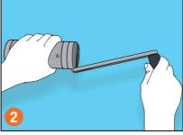
Lift crank arm and slot into groove on top cap. Holding the unit with one hand, begin turning crank in a forwards direction
