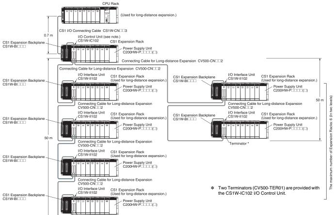
**Note:** If even one Long-distance Expansion Connecting Cable to be used, it is necessary for an I/O Control Unit to be mounted to the CS1 Expansion Rack where the Cable is connected.
