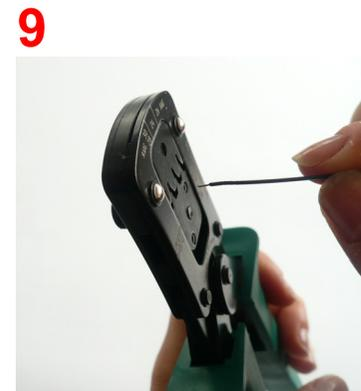
Insert the cable until insulation stop blade.
