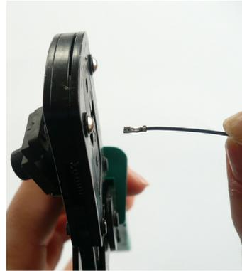
Remove the crimped contact.
