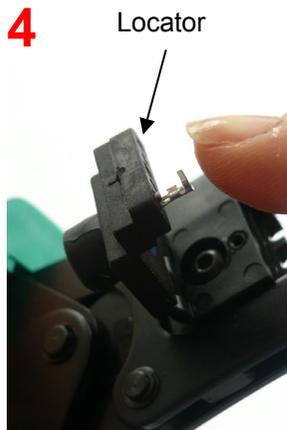
Contact has to be inserted until stop. Please pay attention to the correct cross section.
