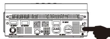
Once the unit has been properly installed and the batteries are connected well, simply press On/Off switch (located on the button of the case) to turn on the unit.
