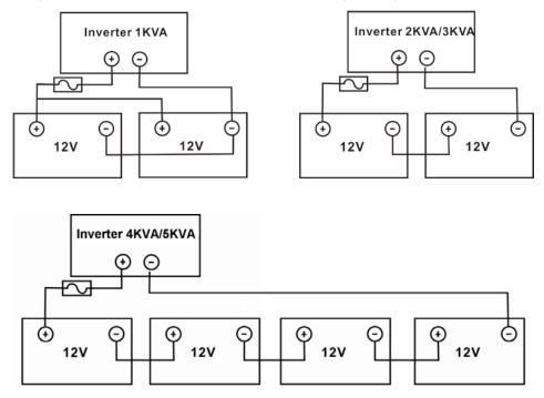
NOTE: Please only use sealed lead acid battery or sealed GEL/AGM lead-acid battery.
