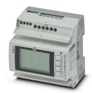
Multi-functional energy measuring device with 24 V DC supply, direct Rogowski connection, and integrated Modbus/TCP interface for measuring electrical parameters in low-voltage installations up to 690 V
