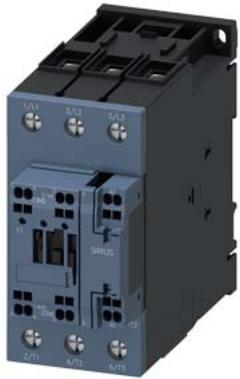
power contactor, AC-3e/AC-3, 41 A, 18.5 kW / 400 V, 3-pole, 20-33 V AC/DC, 50/60 Hz, with integrated varistor, auxiliary contacts: 1 NO + 1 NC, main circuit: screw terminal, control and auxiliary circuit: spring-loaded terminal, size: S2, communication-capable
