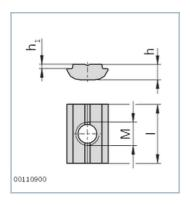
Swivel-in sliding block with spring
