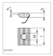
Sliding block, swivel-in, with headless setscrew
