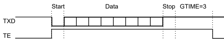
Figure 30-15. Example of TE Drive with Guard Time
