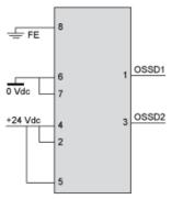
With External Device Monitoring (EDM) feedback loop
