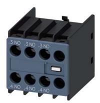
auxiliary switch, on the front, 3 NO, .3/.4, .3/.4, .3/.4, --/-, current path: 1 NO, 1 NO, 1 NO, --, screw terminal, for contactors 3RT2 and contactor relays 3RH2
