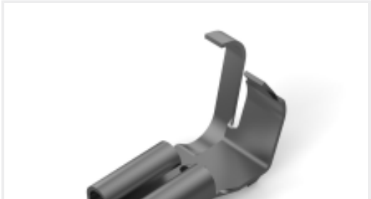
TE Part #170140-6 187 FASTON, FLAG, REC., 16-20 AWG, TPBR
