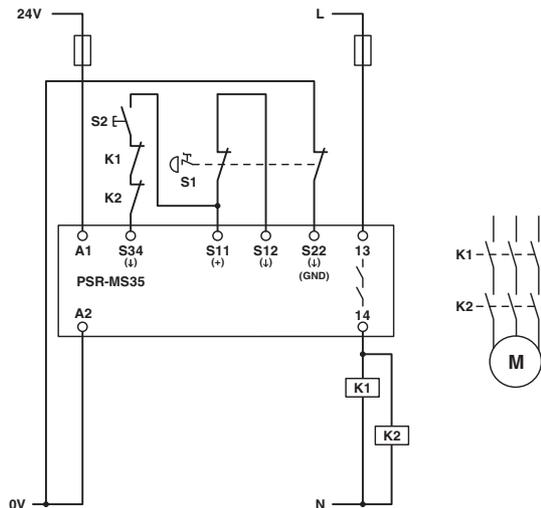
Figure 10 Emergency stop monitoring/manual, monitored start
