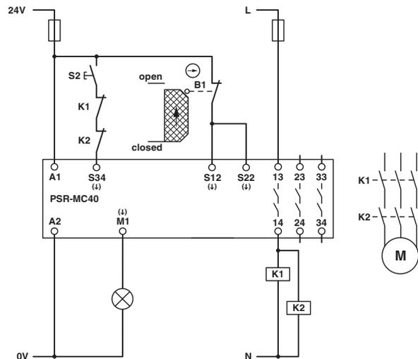
Figure 54 Single-channel safety door monitoring/manual, monitored start
