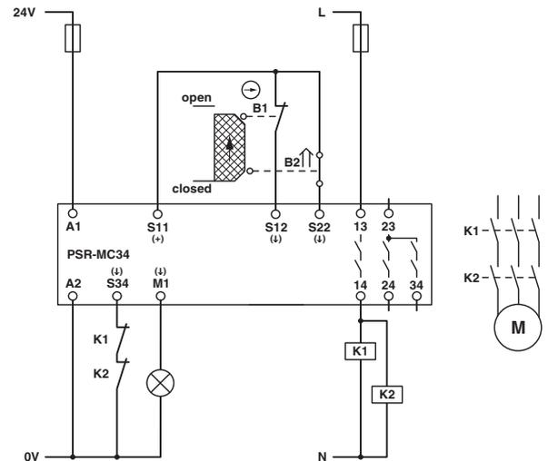
Figure 42 Safety door monitoring/automatic start/without cross-circuit detection
