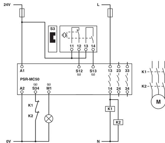
Figure 63 Magnetic switch monitoring/automatic start
