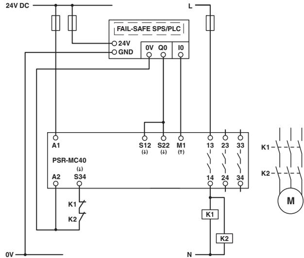
Figure 57 Single-channel connection to failsafe PLC/automatic start
