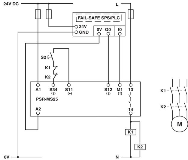
Figure 6 Connection to failsafe PLC/manual, monitored start
