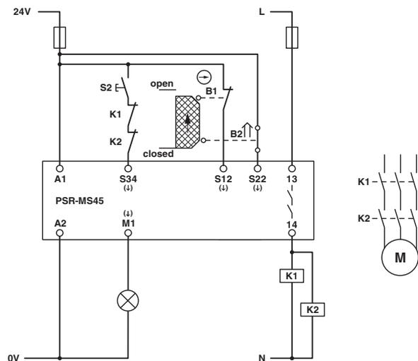
Figure 17 Safety door monitoring/manual, monitored start
