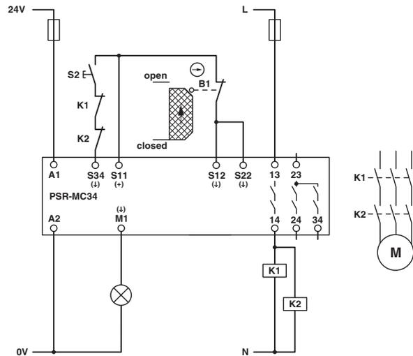
Figure 46 Single-channel safety door monitoring/manual, monitored start
