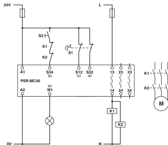
Figure 50 Emergency stop monitoring/manual, monitored start
