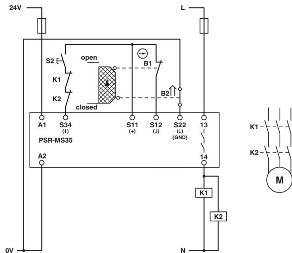
Figure 11 Safety door monitoring/manual, monitored start
