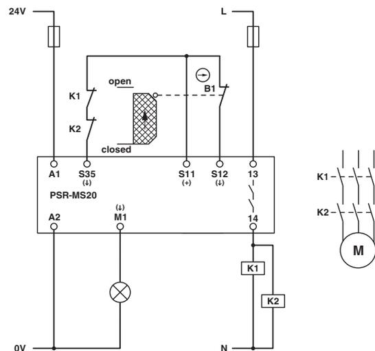
Figure 2 Safety door monitoring/automatic start
