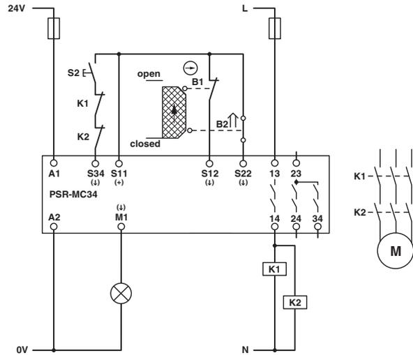
Figure 45 Safety door monitoring/manual, monitored start/without cross-circuit detection
