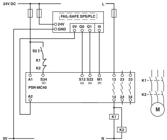
Figure 56 Connection to failsafe PLC/manual, monitored start
