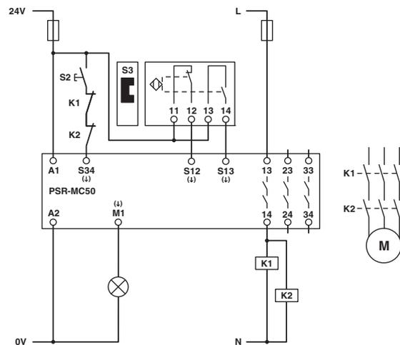
Figure 64 Magnetic switch monitoring/manual, monitored start
