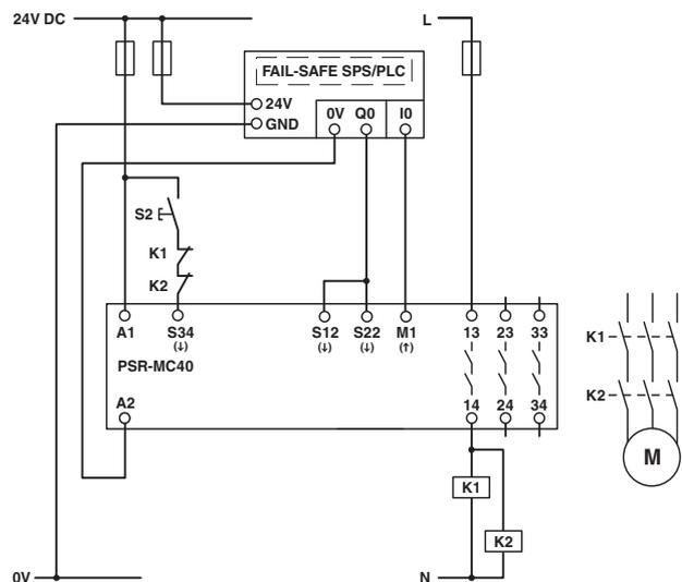
Figure 58 Single-channel connection to failsafe PLC/manual, monitored start
