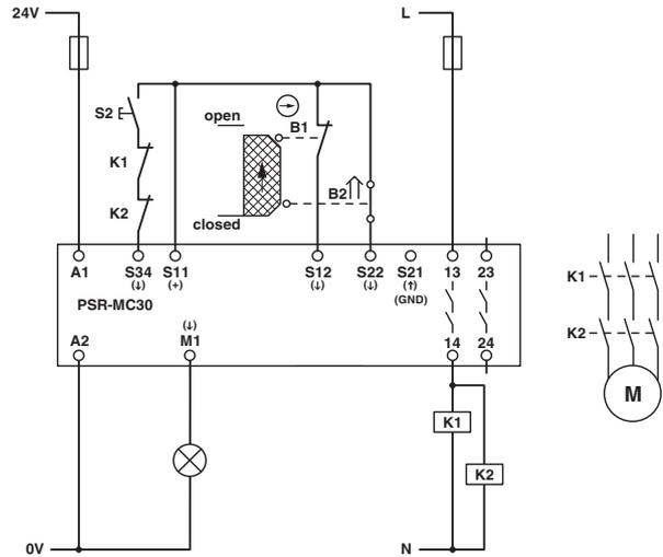
Figure 35 Safety door monitoring/manual, monitored start/without cross-circuit detection
