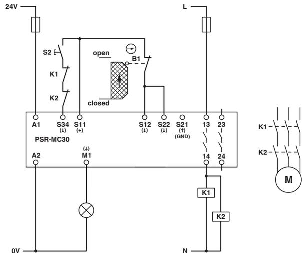
Figure 36 Single-channel safety door monitoring/manual, monitored start
