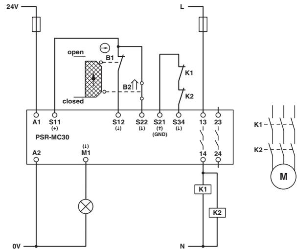
Figure 32 Safety door monitoring/automatic start/without cross-circuit detection
