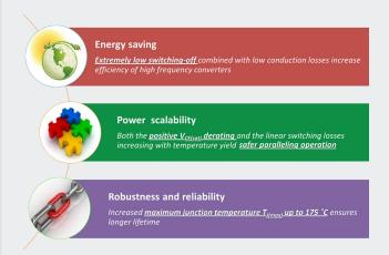
The new "V" family 600V IGBT redefines products in the market, offering the desired trade-off in performance for both hard-switching and soft-switching applications. MOSFET-like dynamic performance during the switch off, earning the "V" family the nickname of "tail-less", produces the key points designers are looking for.
