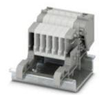
COMBI receptacle, Connection method: Push-in connection, Number of positions: 3, Cross section: 0.14 mm² - 1.5 mm², AWG: 26 - 14, Width: 10.5 mm, Height: 27.1 mm, Color: gray/blue/green-yellow
