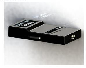
Wi-Fi Digital box streamer is a very innovative device that allows to stream from USB to Wi-Fi all kind of images taken from a digital USB device. It can be used with digital USB microscopes (i.e. Dino-Lite) but even with other devices like USB endoscopes or USB eyes. It breaks the conception of traditional USB digital microscope to realize the following functions: measurement, conservation, copy and transfer of images and video which are difficult for a traditional microscope.
