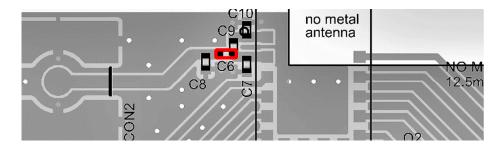
Figure 5: Capacitor connection to external antenna
