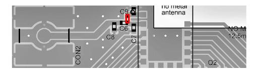
Figure 4: Capacitor connection to internal antenna
