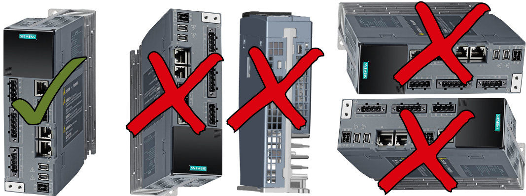
Figure 5-2 Mounting position of the converter
