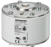
SITOR fuse link, with female thread on both sides, NH3, In: 500 A, aR, Un AC: 1250 V, Un DC: 440 V, front indicator
