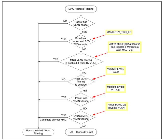
Figure 7.3. VLAN Filtering
