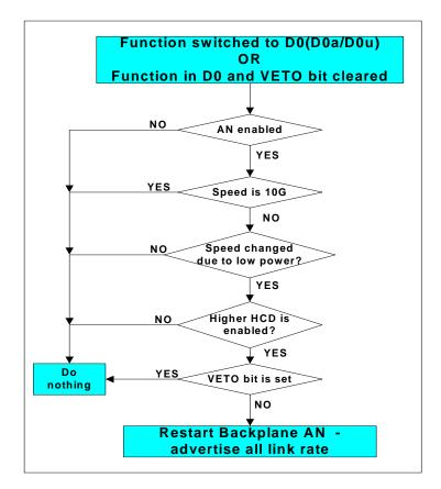
Figure 3.28. MAC Speed Change on Entering Power-up Mode
