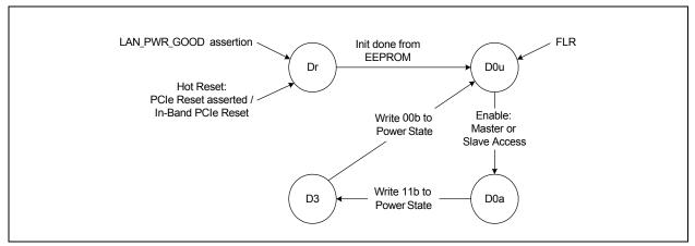
Figure 5.1. Power Management State Diagram
