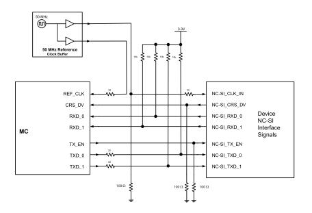
Figure 12-19. NC-SI Connection Schematic: Single-Drop Configuration
