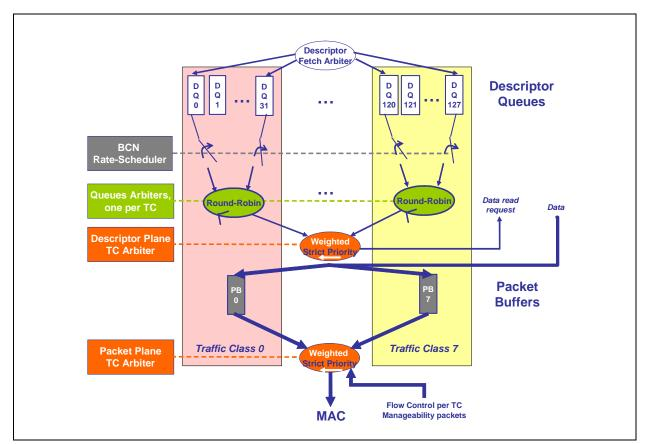
Figure 7.17. Transmit Architecture DCB-on/VT-off — Eight TCs Mode
