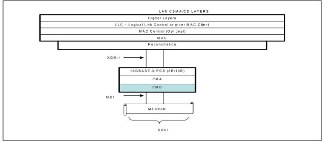
Figure 3.13. Architectural Positioning of XAUI
