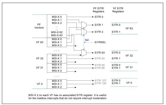
Figure 7.28. PF / VF MSI-X Vectors Mapping to EITR
