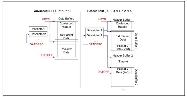
Figure 7.45. RSC — Header and Data Buffers
