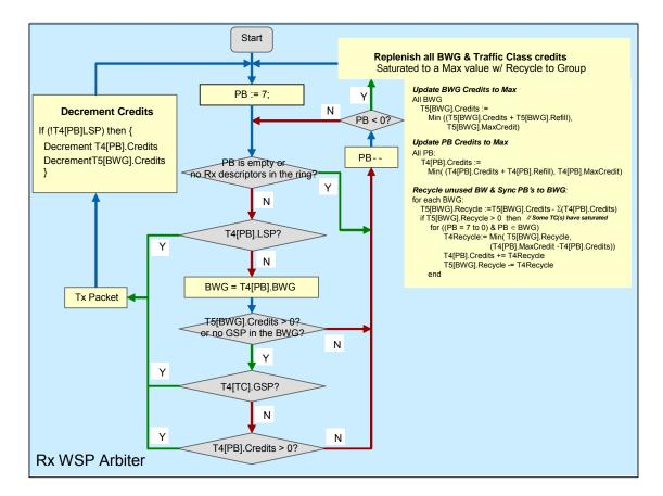
Figure 7.35. Rx Packet WSP Arbiter Operation
