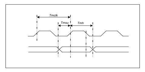
Figure 11.9. MDIO Input AC Timing Diagram
