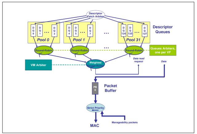
Figure 7.18. Transmit Architecture DCB-off/VT-on - 32 VFs
