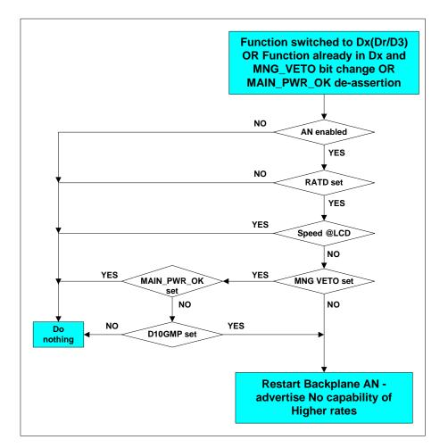
Figure 3.27. MAC Speed Change When Entering Power Down Mode
