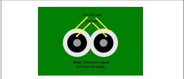
Figure 12-14. Better Differential Signals Via Anti-Pads
