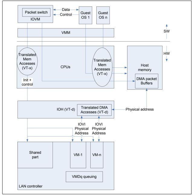
Figure 7.38. System Configuration for Next Generation VMDq Mode
