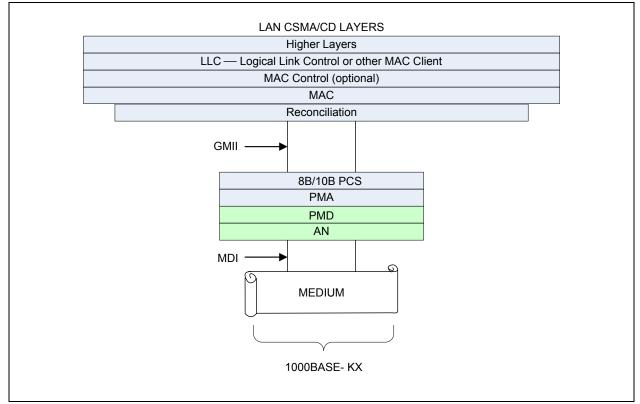
Figure 3.18. Architectural Positioning of 1000BASE-KX
