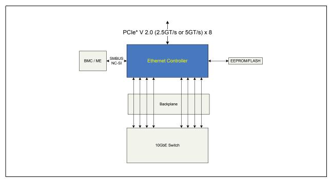
Figure 1.2. Typical Blade System Configuration
