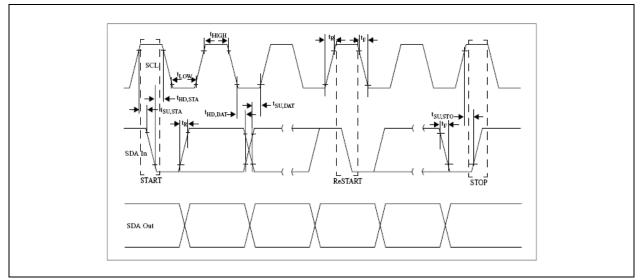
Figure 11.4. SMBus I/F Timing Diagram
