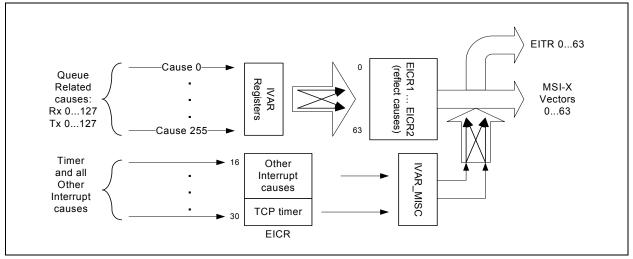
Figure 7.23. Cause Mapping in MSI-X Mode (non-IOV)
