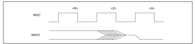
Figure 3.24. Behavior of MDIO During TA Field of a Read Transaction
