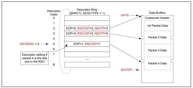
Figure 7.43. RSC Functionality (No Header Split)
