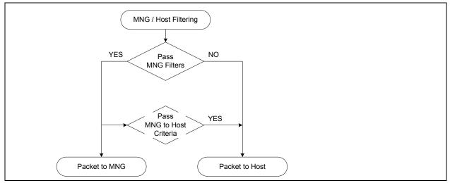
Figure 7.4. Manageability / Host Filtering
