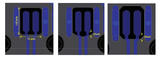
Figure 12-16. Voiding the Reference Planes Under the SFI + Connector Pin Solder Pads
