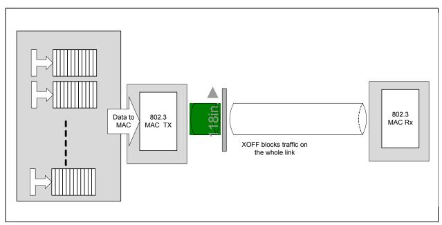
Figure 3.25. 802.3X Link Flow Control (PAUSE)
