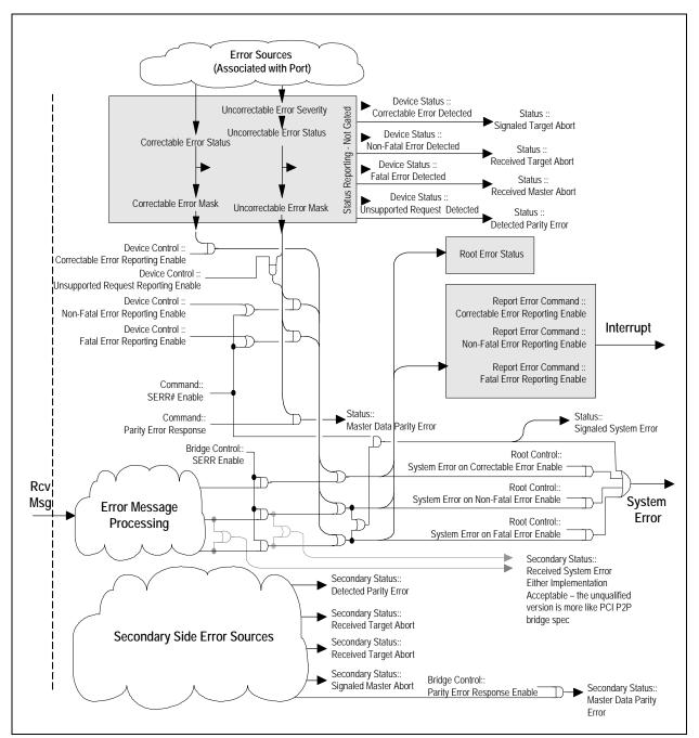
Figure 3.6. Error Reporting Mechanism
