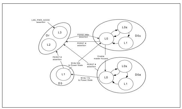
Figure 5.2. Link Power Management State Diagram
