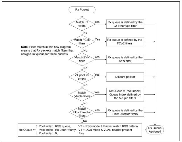
Figure 7.7. Rx Queuing Flow (Virtualization Case)
