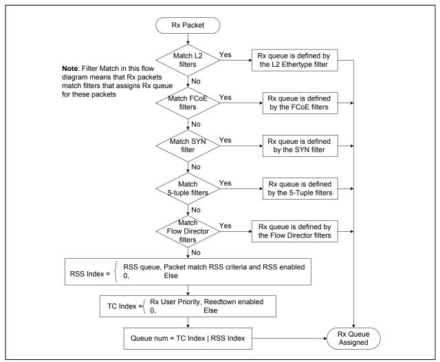
Figure 7.6. Rx Queuing Flow (Non-Virtualized)
