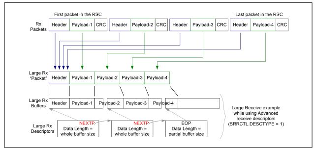
Figure 7.42. RSC Functionality (No Header Split)
