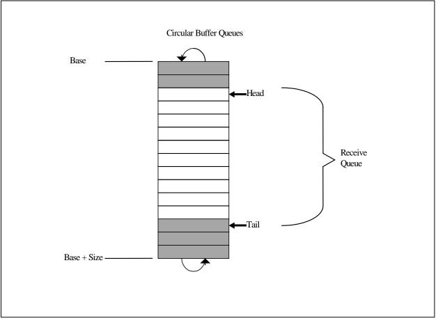
Figure 7.11. Receive Descriptor Ring Structure
