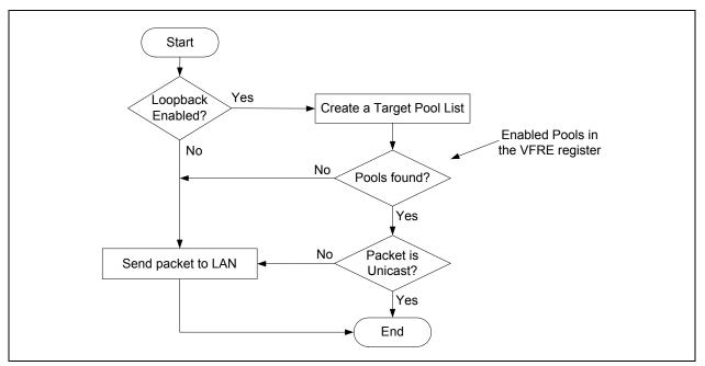
Figure 7.41. Tx Filtering
