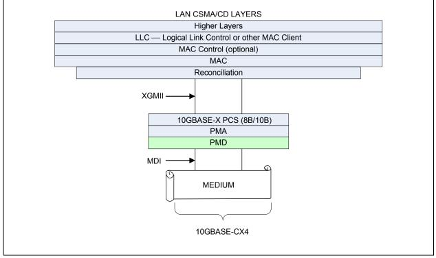
Figure 3.16 shows the architectural positioning of 10GBASE-CX4.
