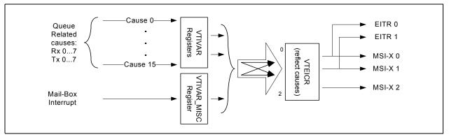
Figure 7.24. VF Interrupt Cause Mapping (MSI-X, IOV)
