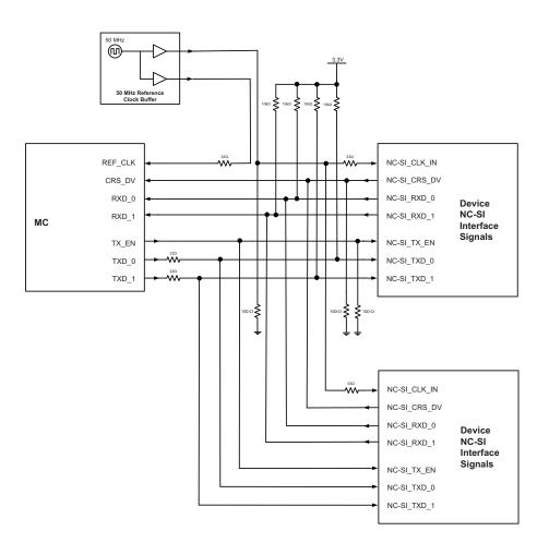
Figure 12-20. NC-SI Connection Schematic: Multi-Drop Configuration
