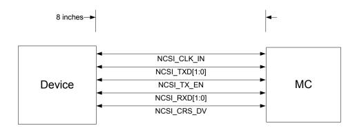
Figure 12-21. NC-SI Trace Length Requirement for Direct Connect
