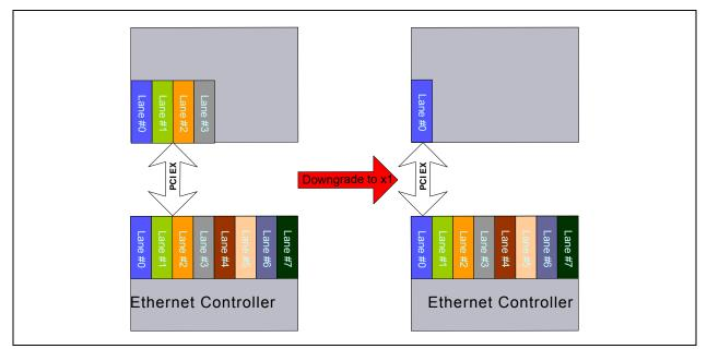
Figure 3.4. Lane Downshift in a x4 Configuration
