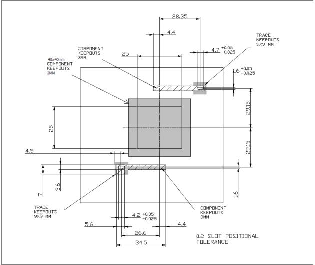
Figure 13-2. Heatsink Keep-out Restrictions
