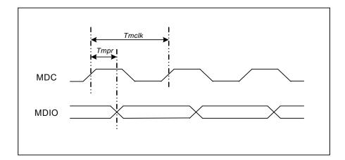
Figure 11.10.MDIO Output AC Timing Diagram
