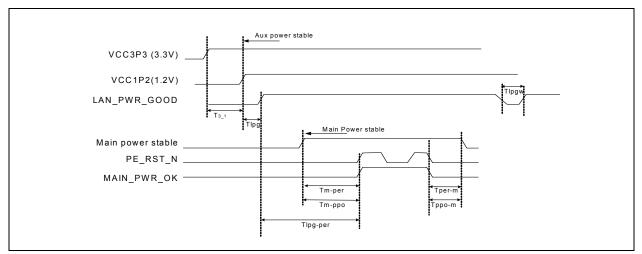
Figure 11.1. Power and Reset Sequencing
