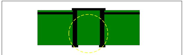
Figure 12-4. Incorrect Via Usage
