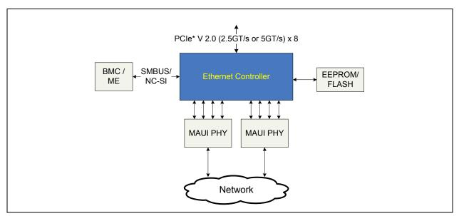
Figure 1.1. Typical Rack / Pedestal System Configuration
