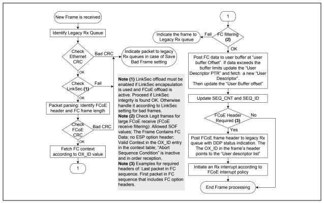
Figure 7.52. FCoE Large Receive Flow Diagram
