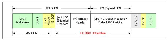
Figure 7.48. FCoE Frame and Relevant Transmit Descriptor Parameters
