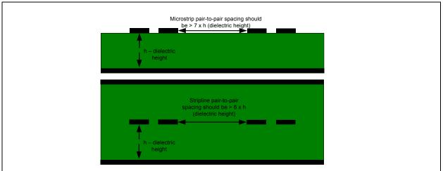
Figure 12-1. Differential Pair Spacing
