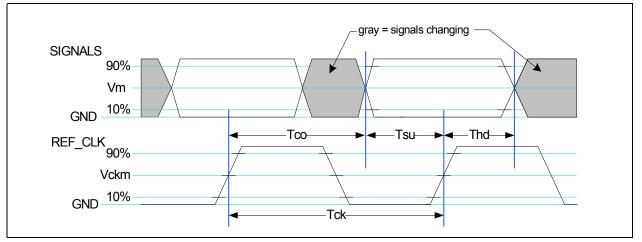
Figure 11.7. NC-SI AC Timing Diagram
