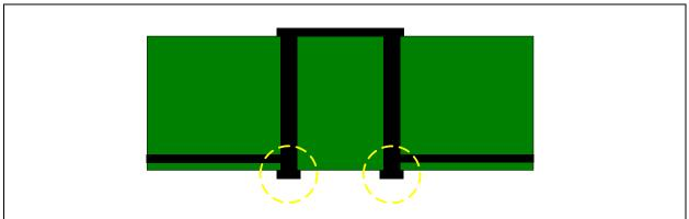
Figure 12-3. Correct Via Usage
