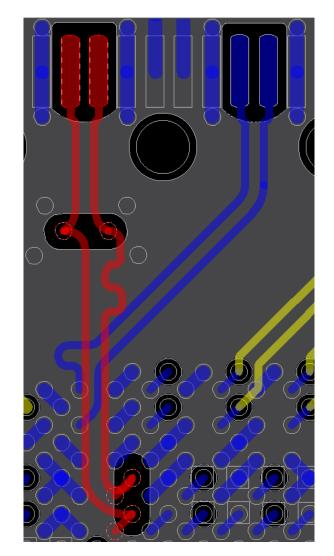
Figure 12-17. SFI + Breakout and Routing Example From the 82599 to SFI + Connector Pad
