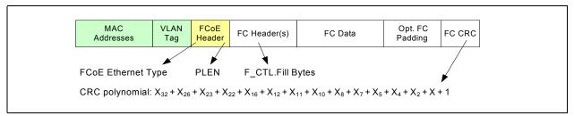
Figure 7.50. Relevant FCoE and FC Fields for CRC Receive Offload
