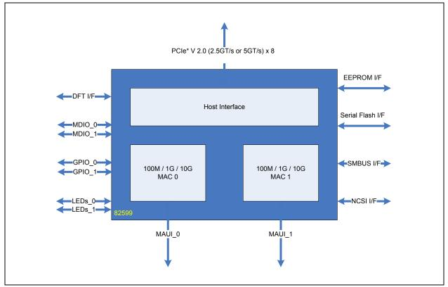
Figure 1.3. 82599 External Interfaces Diagram
