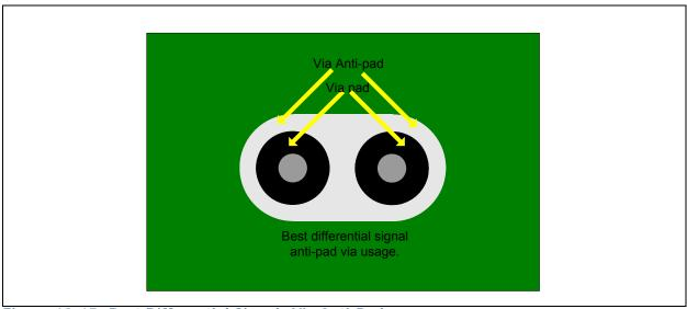
Figure 12-15. Best Differential Signals Via Anti-Pads
