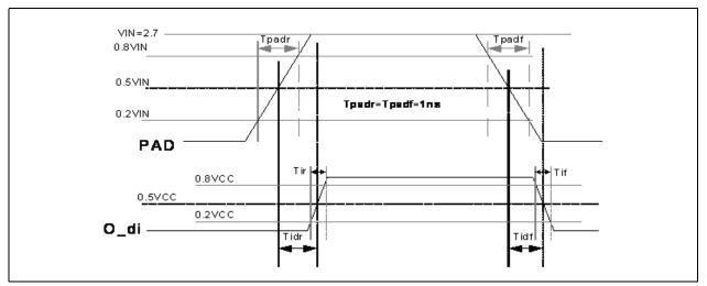
Figure 11.3. Digital 3.3V I/O Input Timing Diagram
