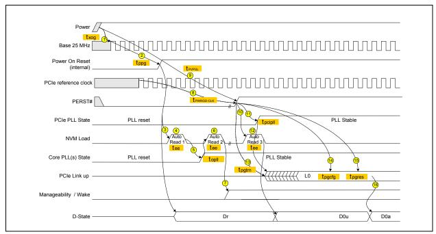
Figure 4.2. Power-Up Timing Diagram
