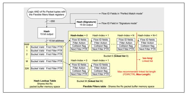
Figure 7.9. Flow Director Filters Block Diagram
