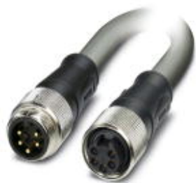
Power cable, 5-position, PVC, Gray RAL 7001, Plug straight 7/8"-16UNF, A-coded, on Socket straight 7/8"-16UNF, A-coded, Cable length: 0.6 m, 2.5 mm 2 conductor cross section, For power supply
