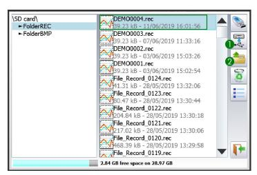
Then, the newly created file can be sent to a USB key (1) or opened on the Data Acquisition System (2) for viewing.
