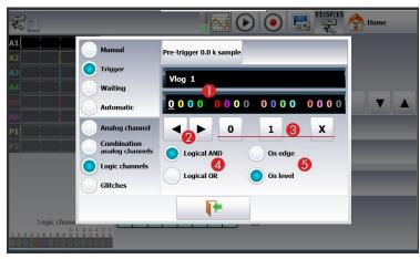
This mode is used to triggers according to the values of the logical channels.
