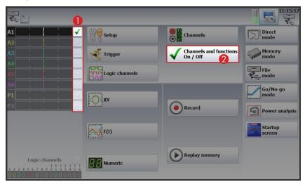
Then, the setting of a channel is done either by directly pressing the channel (1), or by going through the menu "Channels" then pressing the channel concerned (2).
