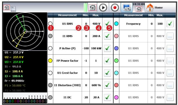
Each measurement or calculation is configured in this table, each line refer to the adjusting of a measurement.
