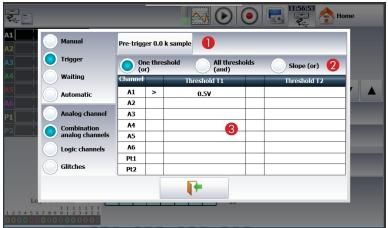
This mode allows, unlike the "Analog Channel" mode, to take into account several analog channels simultaneously.
