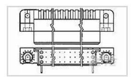
PCB Connector Type: PCB Mount Receptacle
