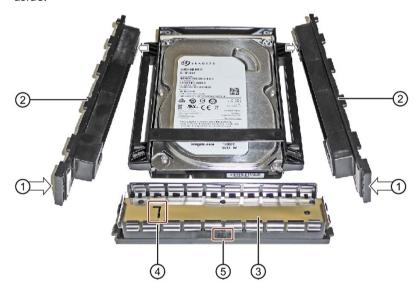
6. Remove the left and right drive mounting bars ② and the drive cover③ from the drive.
