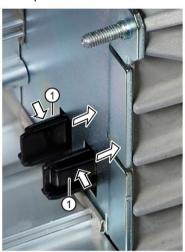
4. Remove the cover ② upwards at an angle at the front of the device.
