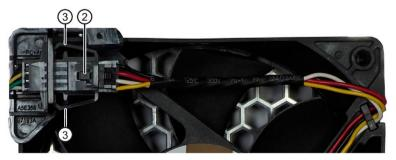
7. Press on the side of the clips ③ and loosen the adapter plug from the cable holder.
