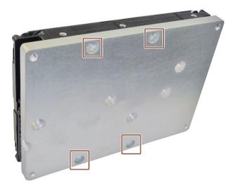
2. Screw from outside the drive bay plate on the inside to the side panel of the enclosure, at position ① or position ②. The SATA connections each lie in the middle ③.
