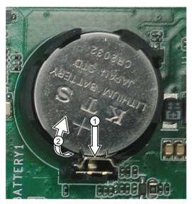
The battery is unlocked and disengages from the socket.
