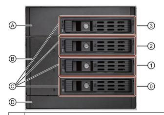
(0) Mounting location 0 for: 2.5" drive in removable tray • 3.5" drive in removable tray (1) Mounting location 1 for: • 2.5" drive in removable tray 3.5" drive in removable tray (2) Mounting location 2 for: • 2.5" drive in removable tray • 3.5" drive in removable tray (3) Mounting location 3 (5.25" tray) for: 5.25" mounting frame with removable tray for 2.5" and 3.5" drives 5.25" drive or 5.25" component Cover of the mounting frame for removable tray (Page 108) (A) (B) Cover
