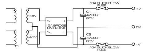
T1 = 450VA 45-0, 45-0 C1/C2 = 4700uF 80V ELECTROLYTICS BRIDGE = 15A 400V PIV THE MAINS INPUT PRIMARY MUST BE PROTECTED BY A HBC CERAMIC FUSE. A 10A RATING IS SUGGESTED.
