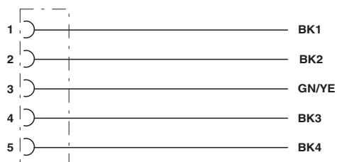
Contact assignment of 7/8" socket
