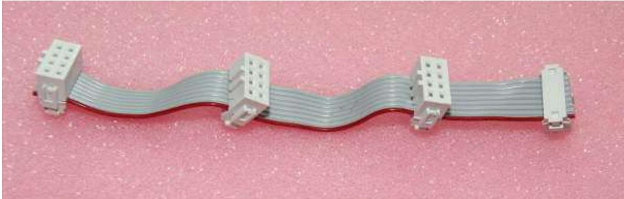
The length of the cable depends on how far apart you want to mount the boards. If you stack them using 15mm stand-offs you need 120 mm cable. You also need an 8-pin IDC press connector per board. I put a video on YouTube how to make a press connector a while ago:
