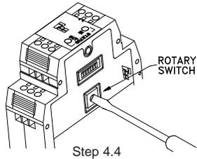
6.3 Press the push-button to enable the rotary switch. The Green input LED now blinks at a faster rate, indicating that calibration values are accessible.
