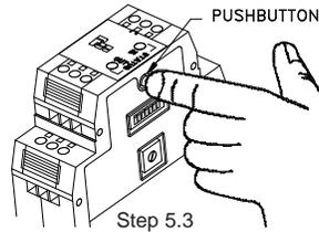
5.3 Press the push-button. The Green input LED blinks rapidly. Maximum Response Time setting is now accessed.
