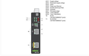
This device is an industrial PoE injector with two Gigabit ETHERNET ports. An ETHERNET port (IEEE 802.3 af/at/bt/4PPoE) provides power to PoE (Powered over Ethernet) devices with up to 71 W. The power output of the PoE injector (Power Sourcing Equipment) is up to 90 W. Additionally, automatic transmission rate detection (auto-negotiation) and automatic detection of the transmit and receive lines (Auto MDI-X) allow simple plug-and-play operation.
