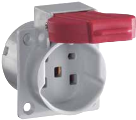
THERMOPLASTIC SOCKET OUTLET 16 A 400 V flush mounting acc. to SEV 5932 type 25 with seal in hinged lid
