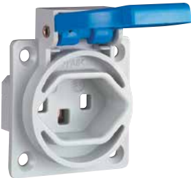
THERMOPLASTIC SOCKET OUTLET 16 A 250 V flush mounting acc. to SEV 5934 type 23 with seal in hinged lid
