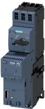
intelligent load feeder direct starter standard 1.2-12 A up to 690 V AC type of coordination 1 frame size S00 for ET 200SP system consisting of 3RC7140-1KE00, 3RV2311-1KC20, 3RT2017-2BB42
