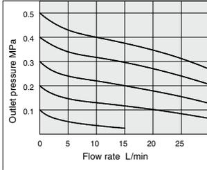
Conditions/ Inlet pressure: 0.7 MPa, Outlet pressure: 0.2 MPa, Flow rate 2 L/min
