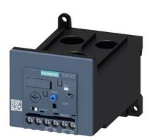
Overload relay 12.5...50 A Electronic For motor protection Size S3, Class 10E Stand-alone installation Main circuit: Straight-through transformer Auxiliary circuit: Screw Manual-Automatic-Reset
