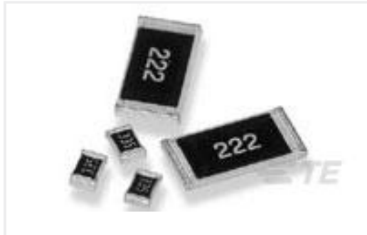
TE Part #1623097-3 CRG0805 1% 10K 10K RL
