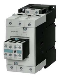
CONTACTOR, AC-3 30 KW/400 V, DC 24 V, 2 NO + 2 NC 3-POLE, SIZE S3, SCREW CONNECTION
