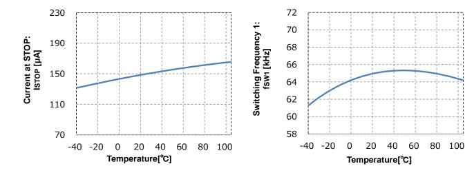
Figure 20. Current at STOP vs Temperature
