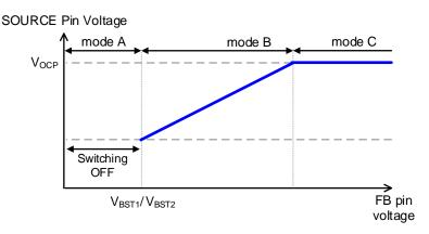
Figure 5. State Transition of SOURCE Pin Voltage by FB Pin Voltage
