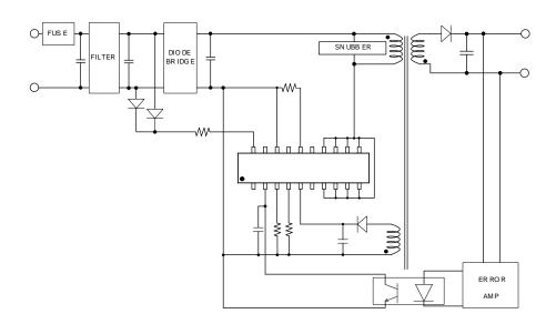
Figure 16. Flyback Application Diagram
