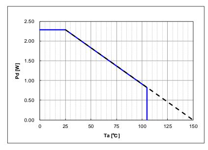
Figure 15. SOP20A Thermal Dissipation Characteristic
