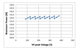
Figure 9.<sup>(Note 2)</sup> Example of Maximum Power ( $L_p = 450 \mu H, R_s = 0.22 \Omega$ )
