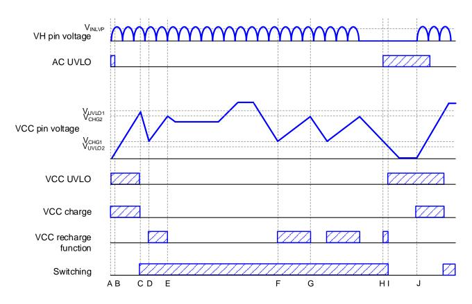
Figure 3. Timing Chart of VCC UVLO and VCC Recharge Function
