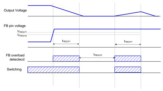
Figure 7. FB Overload Protection Function
