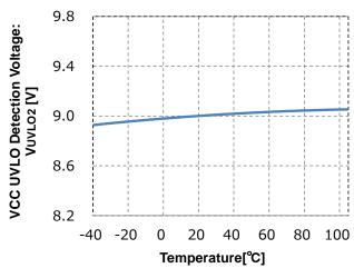
Figure 22. VCC UVLO Release Voltage vs Temperature
