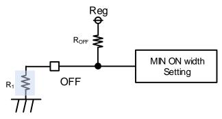
Figure 12. OFF Setting Circuit
