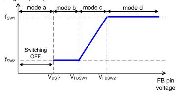
Figure 4. State Transition of Switching Frequency
