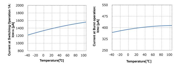
Figure 18. Current at Switching Operation 1A vs Temperature
