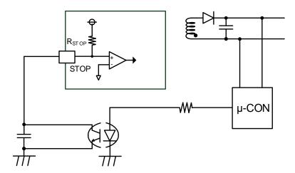
Figure 14. External Stop Circuit
