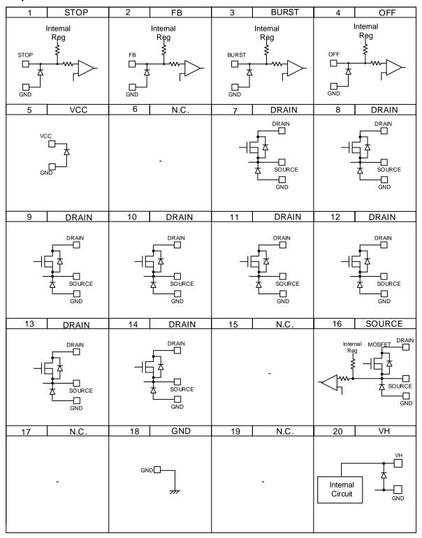
(Note) The N.C pin must be open on the board. It means not to connect GND etc.
