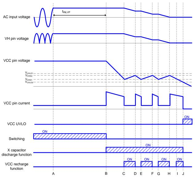
Figure 2. Timing Chart of X Capacitor Discharge Function
