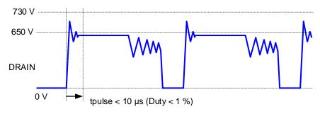
Figure 17. DRAIN pin Ringing Waveform
