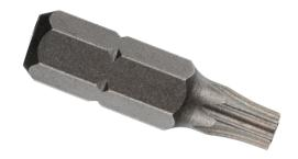
RS Pro Torx Tamper screw bits are a safety profile bit which prevents unauthorised persons from screwing in and out. It follows the normal Torx profile but there is an added bore hole in the tool which corresponds with the additional pin on the screw head. Supplied in a compact plastic box.
