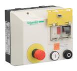
Enclosed DOL starter, TeSys LJ, 2.5-4A,24V AC coil, including 1 LC1K, GV2ME, with integral transformer, 2 pushbuttons, padlocking
