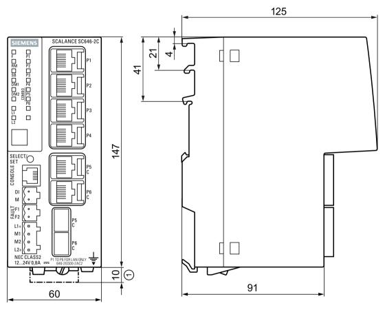
Figure 9-1 Front view and side view of the SCALANCE SC646-2C. All SCALANCE SC-600 modules have the same dimensions.
