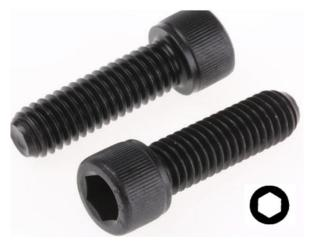
Socket Caps have a small cylindrical head with tall, vertical sides giving them space saving advantages as well as greater tensile strength. They also require less side room for wrenches. These socket screws are used in many applications including the manufacture and repair of vehicles, machine tooling, tools and dies, machine production and repair and general engineering applications. Most importantly, socket cap head screws provide safety, reliability and cost efficiency.
