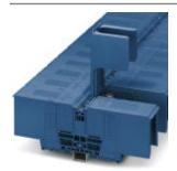
Bolt connection terminal block, Connection method: Bolt connection, Number of positions: 1, Cross section: 25 mm² - 300 mm², AWG: 4 - 600, Width: 54.8 mm, Color: blue, Mounting type: NS 35/7,5, NS 35/15, ct screw connection
